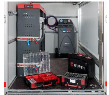
Everything on board e.g. shelf system, ORSY case, COOLIUS A/C service unit
